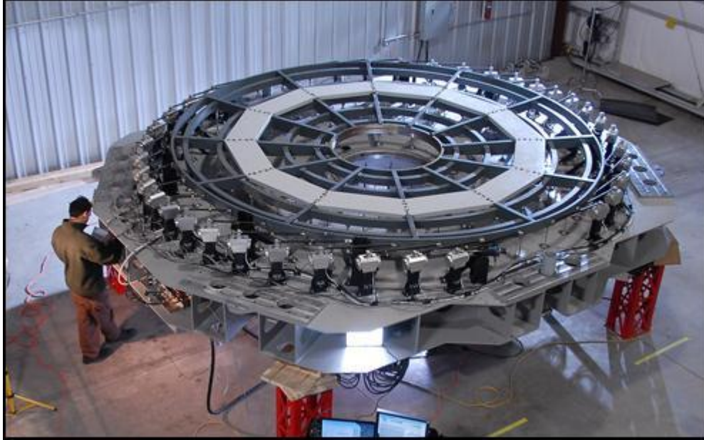
Figure 1. AOS M1 assembly and testing with mirror simulator
