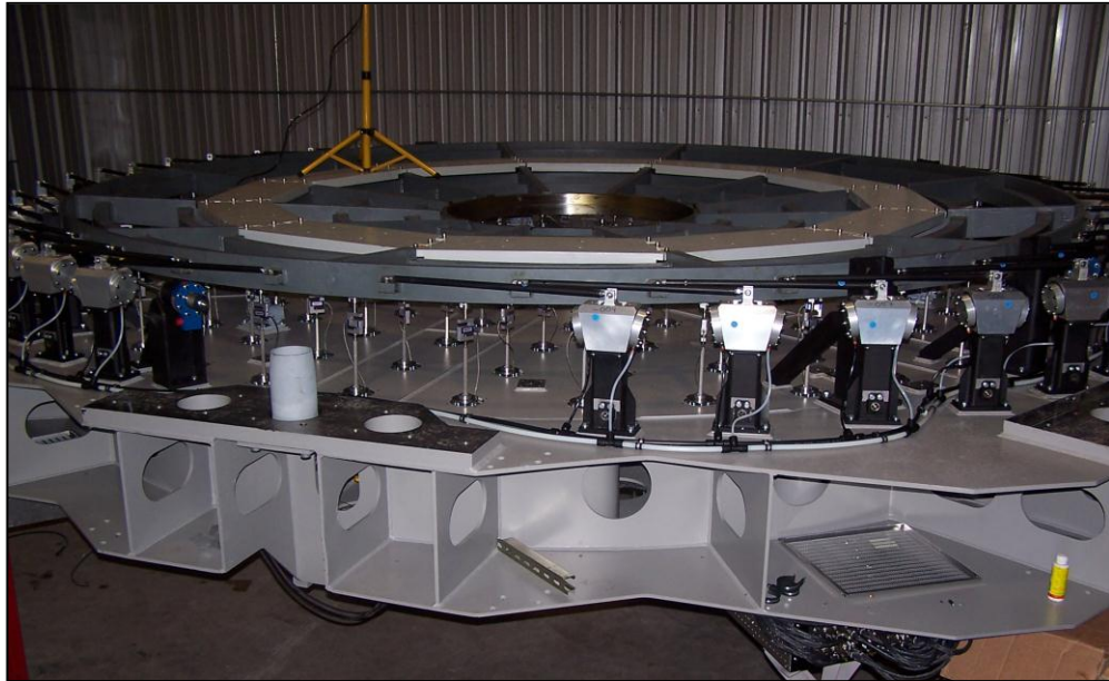
Figure 19. Mirror Supports Installation on M1 Cell
