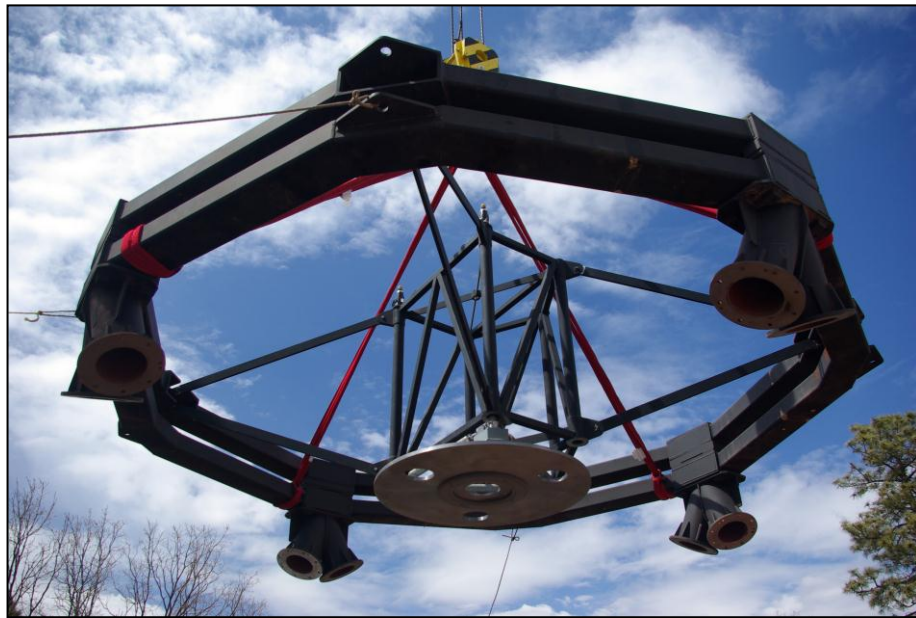
Figure 21. M2 Top End showing M2 frame and simulator
